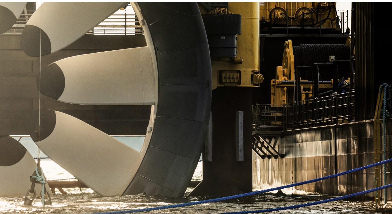
A marine current power underwater turbine on a test platform. ^
